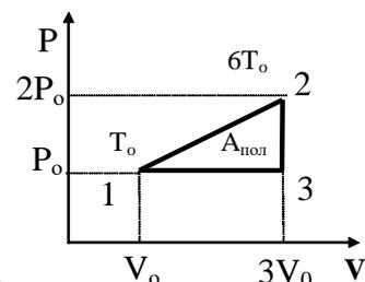
$$A_{\text{полезн}} = \frac{1}{2} \Delta P \cdot \Delta V = \frac{1}{2} (2P_0 - P_0) \cdot (3V_0 - V_0) = P_0 V_0 = \nu R T_0;$$
