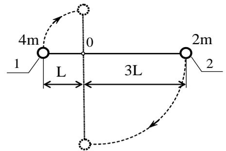
$$\frac{4mv_1^2}{2} + \frac{2mv_2^2}{2} = 2mg \cdot 3L - 4mgL \quad (1)$$
