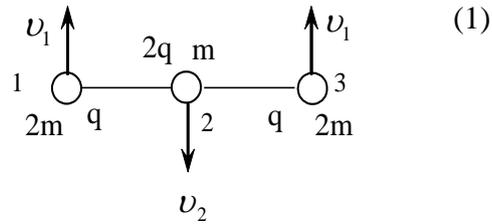
$$2) \quad 2 \frac{2m v_1^2}{2} + \frac{m v_2^2}{2} = \Delta W_{\text{эл.}}$$
