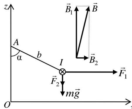
$$\begin{cases} I_1 B_z b \cdot b \cos \alpha_1 - (I_1 B_x b + mg) \cdot b \sin \alpha_1 = 0, \\ I_2 B_z b \cdot b \cos \alpha_2 - (I_2 B_x b + mg) \cdot b \sin \alpha_2 = 0. \end{cases}$$
