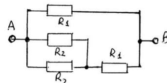
$$R_{AB} = \frac{\left(\frac{R_2}{2} + R_1\right) \cdot R_1}{\frac{R_2}{2} + R_1 + R_1} = \frac{(30 + 30) \cdot 30}{30 + 30 + 30} = 20 \text{ Ом.}$$
