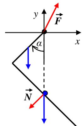
$$\left\{ \begin{array}{l} F_x = N \sin(\alpha) = \frac{12mg}{125} \\ F_y = mg + N \cos(\alpha) = \frac{141mg}{125} \end{array} \right\} \Rightarrow F = \sqrt{F_x^2 + F_y^2} = \frac{3\sqrt{89}}{25} mg.$$
